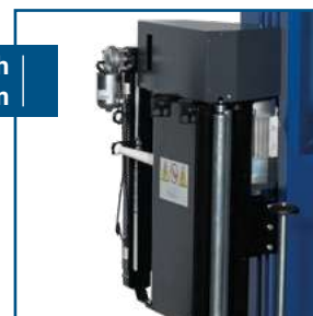
Pps Carriage With Roping System
